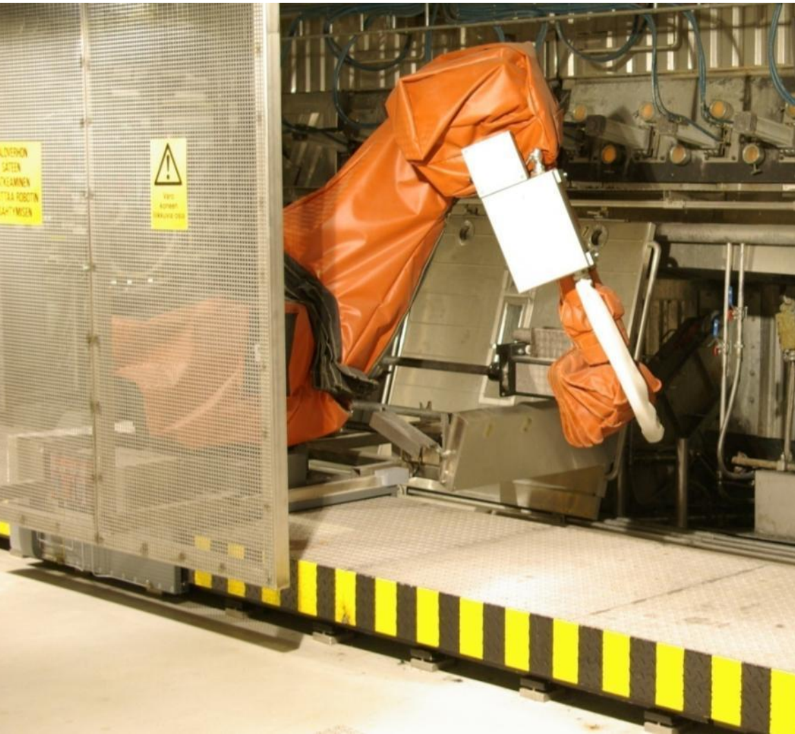
Smelt Spout Robot At Kymi Mill
